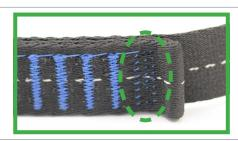
The structural stitch pattern includes a sacrificial bumper stitch pattern which protects the structural bar tack stitches. See highlighted section for bumper stitches. These stitches are allowed to unravel over time due to impacts with the Nozzle. Trim any loose threads in this section. When this section is completely unraveled over time, the entire webbing assembly must be replaced.
